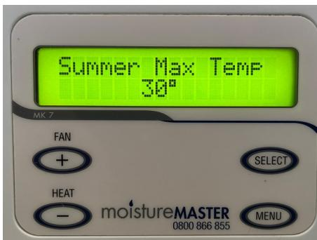
If you do not have the SUMMER BYPASS Option fitted the Fresh Air Supply fan will stop working at the SUMMER MAX TEMP. This will prevent the system from heating your home up on a hot summers day.
