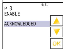
The unit can only be switched on if the contact is closed. If the contact is open, the display will show „NOT ENABLE“. The contact has to be closed and at the end confirmed by selecting „OK“. The default mode is AUTOMATIC.
