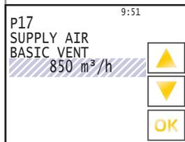
**P 17 Basic ventilation supply air / P 18 Basic ventilation extract air**
