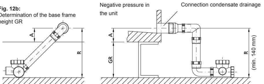
**Example:** Negative pressure at the condensate drain connection  $P=1500 \text{ Pa}$  and distance A is 70 mm.
