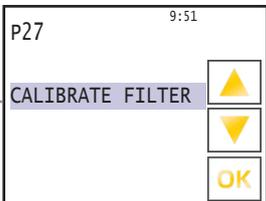
The entire ventilation system has to be complete in order to execute the filter calibration. By touching the icon „▲“, the unit switches to the calibration mode. Display flashes „CALIBRATE FILTER“.
