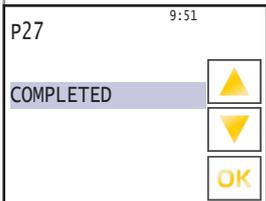
After calibration, the display shows „COMPLETED“.
