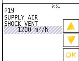
**P 19 Intermittent ventilation supply air / P 28 Intermittent ventilation extract air**
