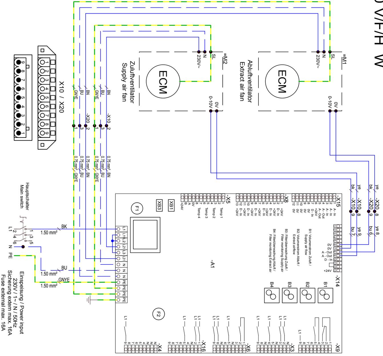
**ETA K 1600** Wiring diagram No.: 137795 Part 1
