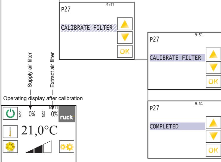
By touching the icon „▲“, the unit switches to the calibration mode. Display flashes „CALIBRATE FILTER“. After calibration, the display shows „COMPLETED“. The contamination display is set back to 0% after calibration mode. The filter change counter will then increase by one.
