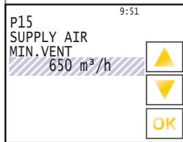
**P 15 Minimum ventilation supply air / P 16 Minimum ventilation extract air**
