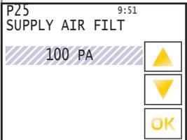
**P 25 Supply air filter pressure loss**
