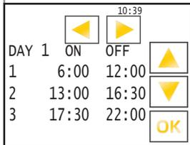
Row (1) flashes on the display, indicating the time when the unit should start on day 1 (Monday) (ON). You can set the hours with „▲“ and „▼“ and then confirm with „▶“. The display then switches to setting the minutes which you can also set with „▲“ and „▼“ and then confirm with „▶“. (The minutes are set in 5-minute increments)
