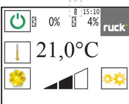
The battery's operating capacity is checked when voltage is applied to the unit. An empty battery is indicated by a battery symbol in the status display.
