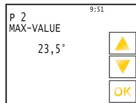
If the desired value is set, you can confirm it with a simple touch. You can further go through the menu with the buttons „▲“ and „▼“ or return to the Operating display with „OK“.
