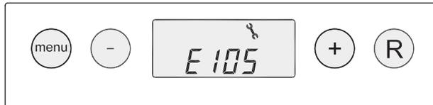
In the event of a locking fault, a fault code will be displayed in addition to the fault symbol, see Display codes on page 39.
