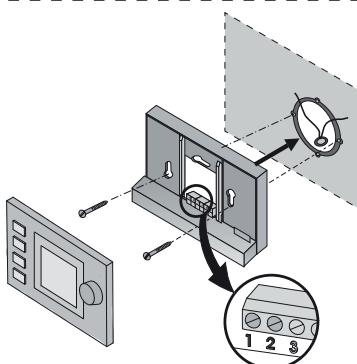
*The optionally available control unit must be connected to this connector eBUS.*
