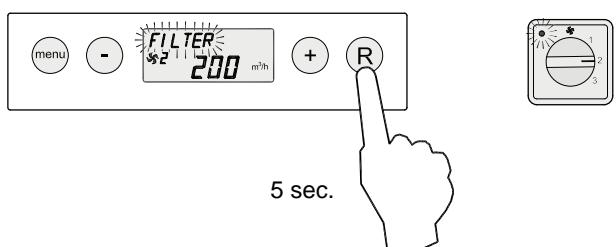
After the filter reset, the text "FILTER"; disappears, the light at the multiple switch is off and the display is back to operating mode.
