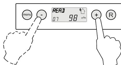
5. Press the 'R' key twice to go back to operating mode. If no key is operated during 5 minutes, the appliance automatically returns to operating mode.
