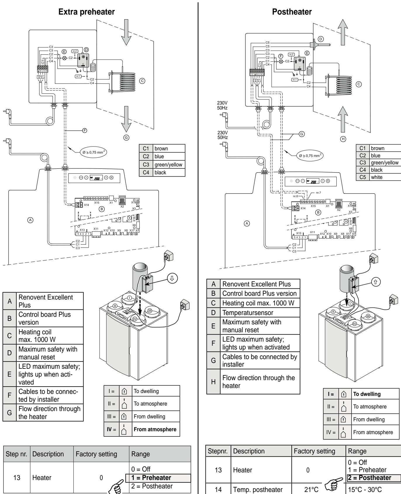
**11.6 Connection example geo heat exchanger (only possible for the Renovent Excellent Plus)**
